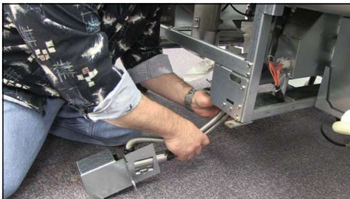
Figure 2: Slip the sensor assembly between the base channel and the right filter rail.
