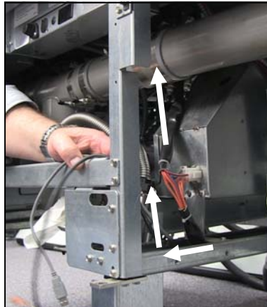
Figure 7: Remove screws on underside of bezel.
