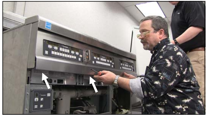
Figure 7: Remove screws on underside of bezel.
