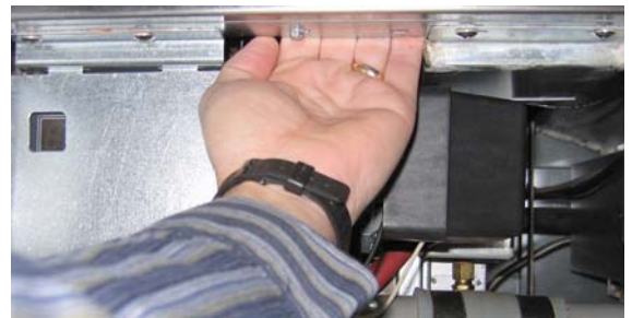
Figure 13: The gas reset switch is on the back side of the control box on the left side of the fryer.
