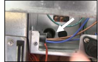
Figure 8-9: Route the harness from the sensor along the base channel and up the vertical cabinet channel (at left). Secure with wire ties. Route the harness through a bushing and into the control box (above).
