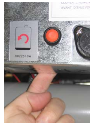
Figure 14: The electric reset switch is under the controller on the right side of the fryer.
