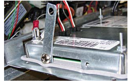
Figure 11: Remove screw and rotate cover to access SD card slot.
