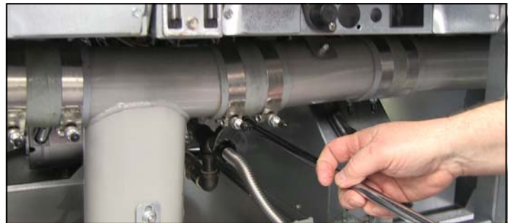
Figure 1: Use a 1 1/16 crow-foot wrench to remove flex line between the pump and the pick up.
